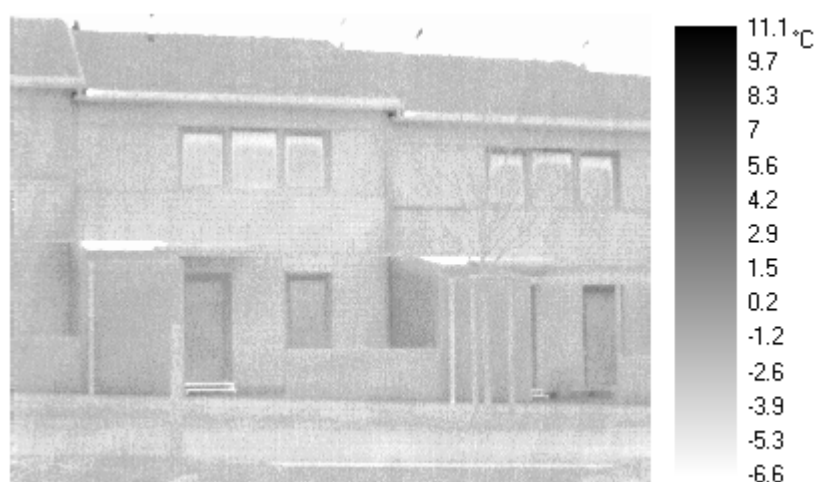
Figure 34: Outdoor thermograph of a section of the houses in row 9 (north side). The area under the roof overhand and under the canopy over the main door seem warmer, since these areas are „covered“ from radiation into the cold night sky. Otherwise, the facades show continuous low temperature of around -4\text{ }^{\circ}\text{C} .
